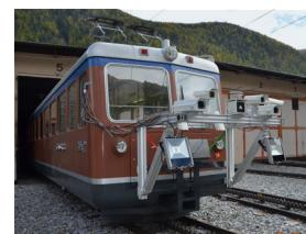
The configuration of the system can be assembled according to customer requirements and can be flexibly mounted on a carrier vehicle. The data is recorded with speeds up to 80km / h. Thus, regular traffic is not disturbed and there is no need for a line closure. We guarantee a maximum benefit with a minimum disturbance of the traffic.
